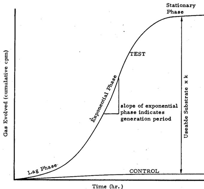
FIG. 1. Labeled release experiment idealized response.
