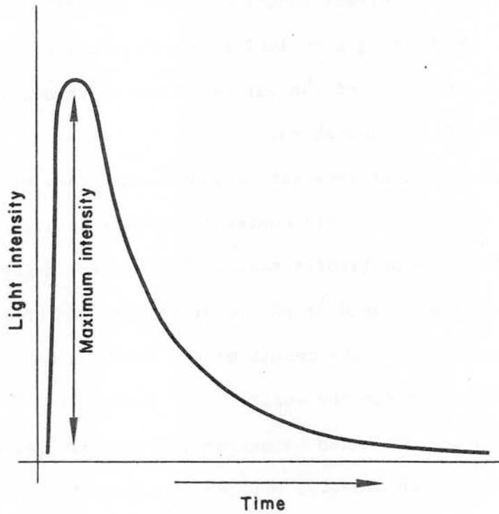
Figure No.1 — A schematic representation of the bioluminescent reaction as recorded by an oscilloscope.
