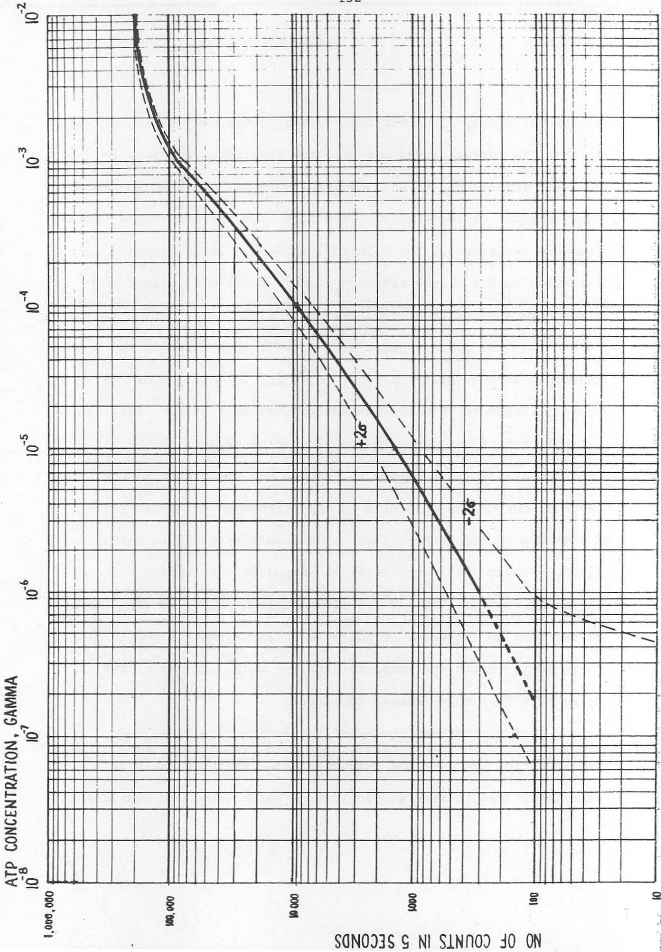
FIG 28 ATP DETECTION SENSITIVITY
